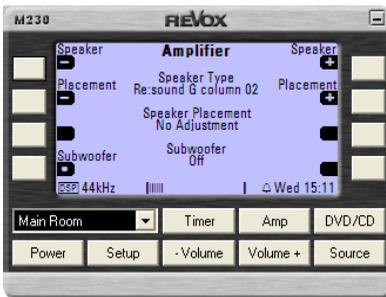
Re:system M100 amplifier menu The basic settings for the amplifier part are made here, including the specific adaptation to the Revox Re:sound speakers.
