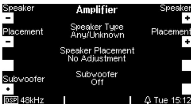
By means of the buttons Speaker +/- you can select your Revox speaker. Should the list not include your speaker from the current speaker range, please make sure that the latest firmware is installed on your M100.
