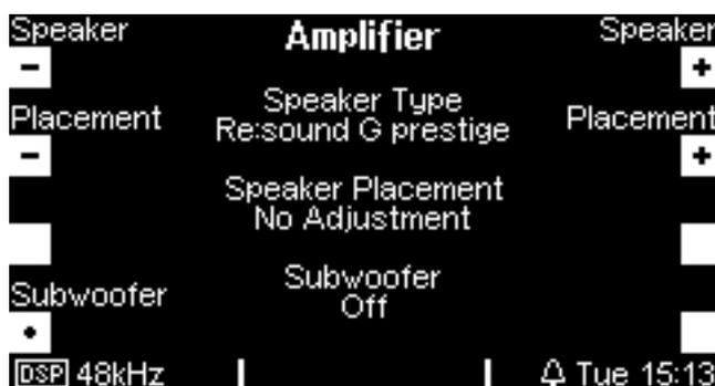
In the next step you can make the adjustment to the placement of the speaker in the room. „No Adjustment“ indicates that the speaker stands in free space.
